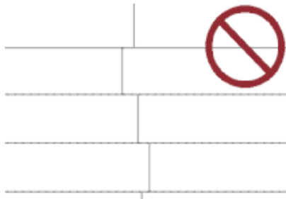
(fig 1) Avoid board-end "line up"
